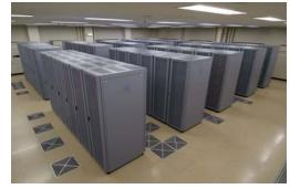
with single core, to provide the best balance between CPU FLOPS and memory bandwidth as well as network bandwidth. The parallel processing network consists of 6-way trunked Gigabit Ethernet in very unique 3-D HyperCrossbar topology.
