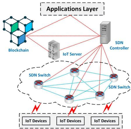
Fig. 1. Conceptual secure IoT design through blockchain and SDN.
