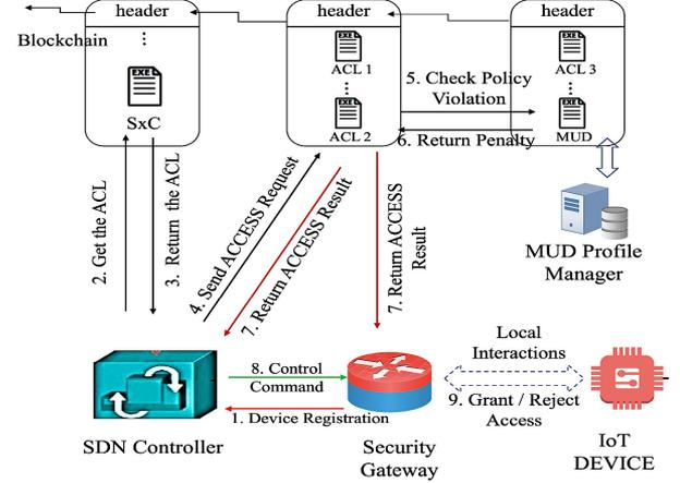
Fig. 10. Blockchain-based smart contract scheme.
