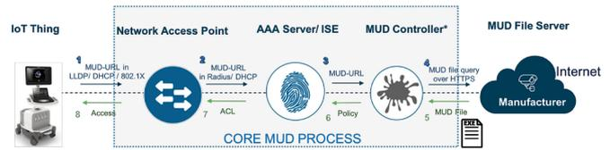
Fig. 2. MUD enabled IoT workflow.
