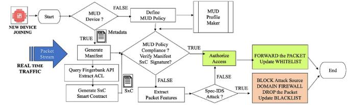
Fig. 11. IoT device joining process.
