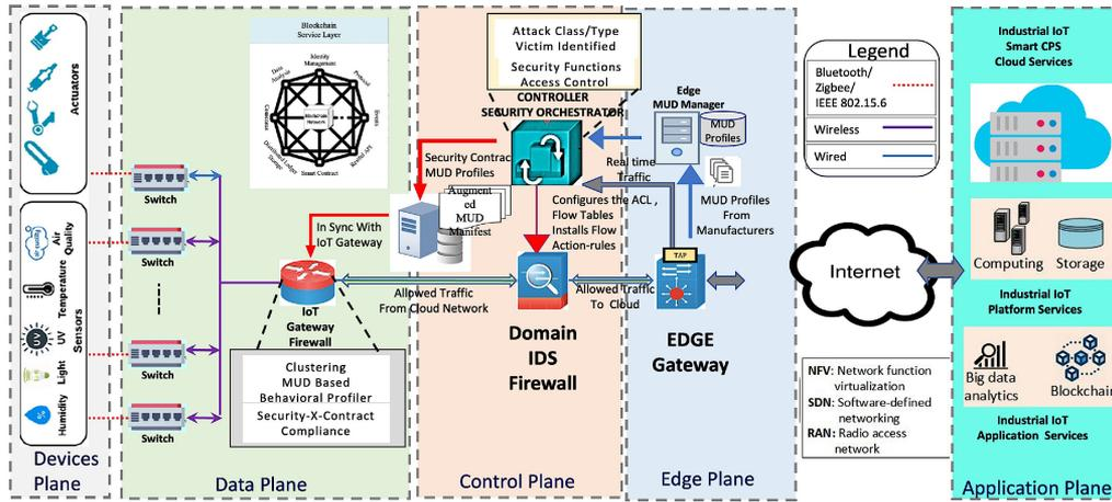
Fig. 5. Proposed software-defined blockchain-based security framework for MUD-Aware industrial-IoT infrastructure.
