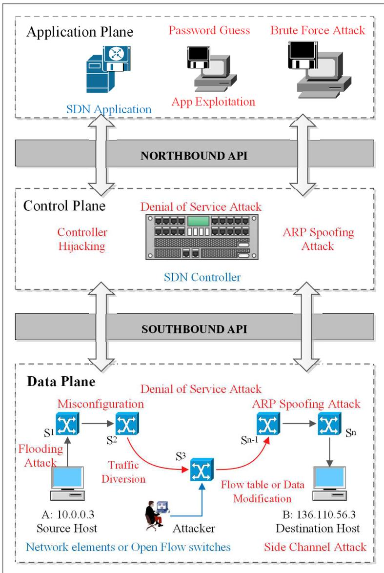
FIGURE 2. Attack vectors at different layers of SDN architecture.
