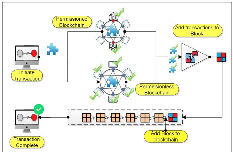
FIGURE 3. Blockchain: the process flow and architecture.
