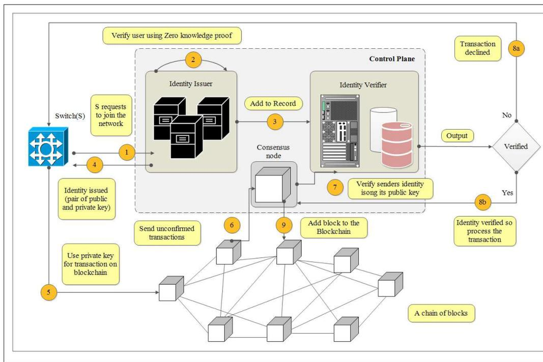
FIGURE 5. Blockchain as a service for switch verification and validation.
