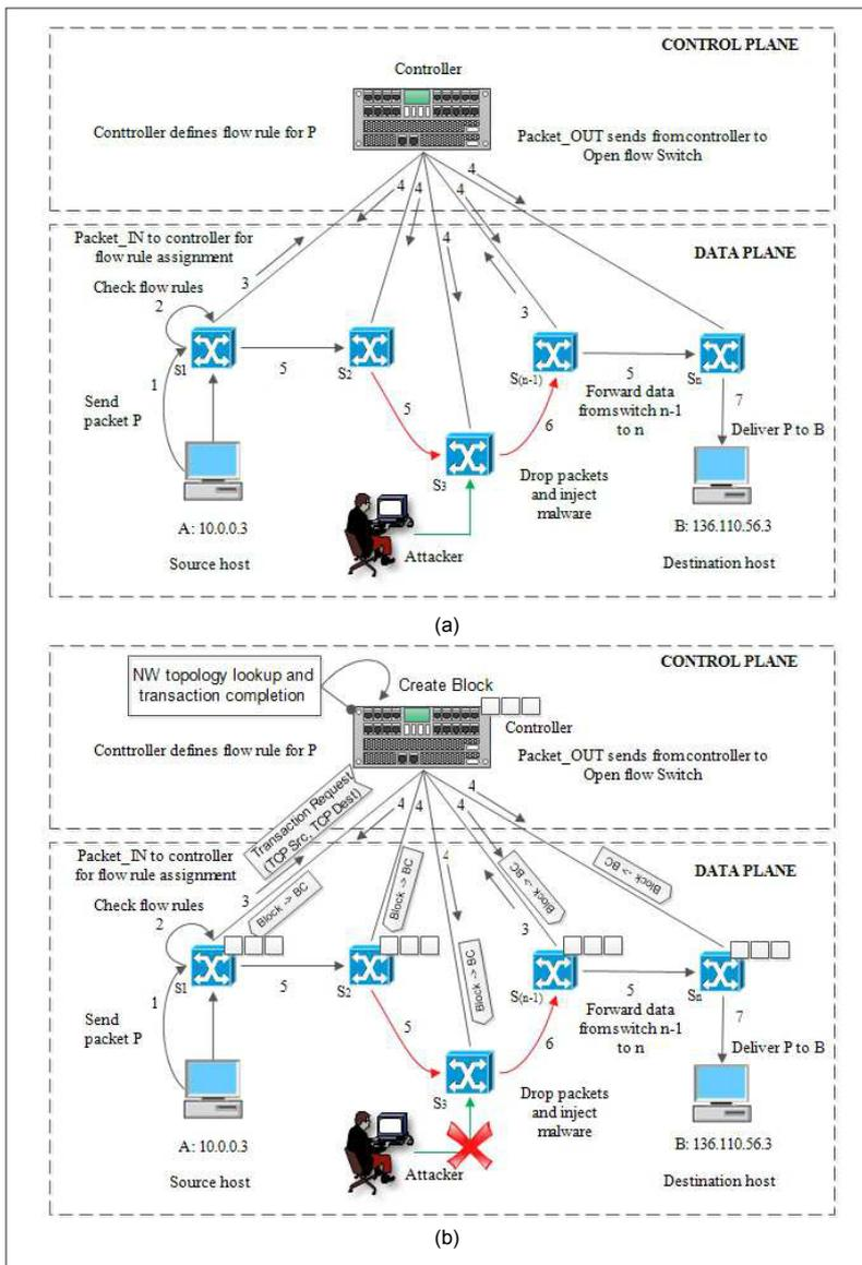
FIGURE 4. Malware-compromised switch in SDN architecture; a) Case1: malware-compromised switch; b) Case2: blockchain as a service for secure traffic flow.
