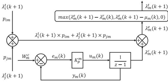
Fig. 3. A part of the feedback control system in QFC.
