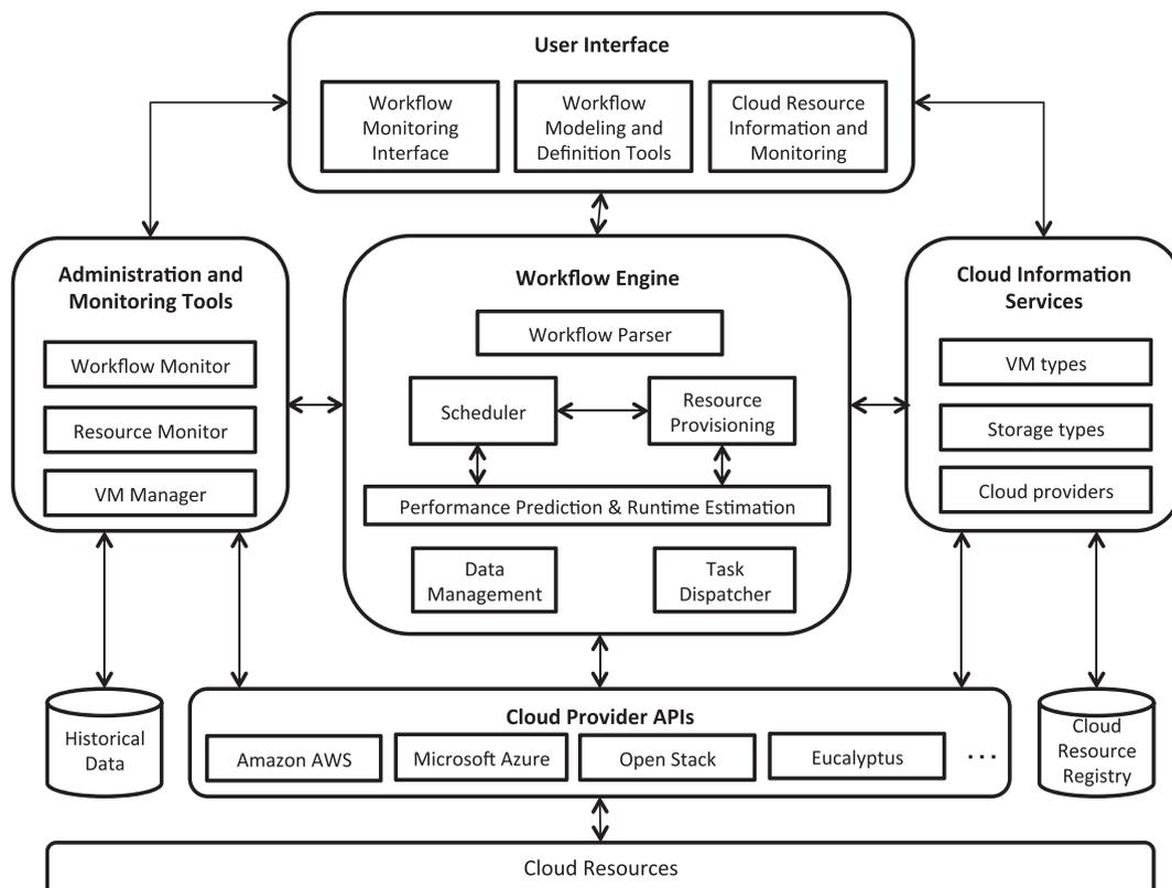
**FIGURE 3** Reference architecture of a workflow management system
