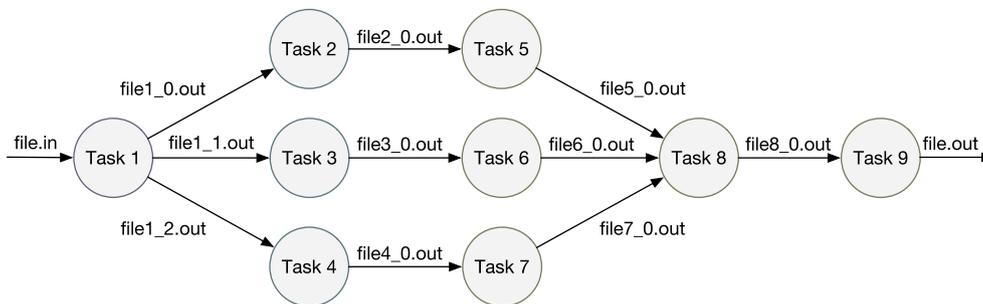
**FIGURE 1** Sample workflow with nine tasks. The graph nodes represent computational tasks and the edges the data dependencies between these tasks
