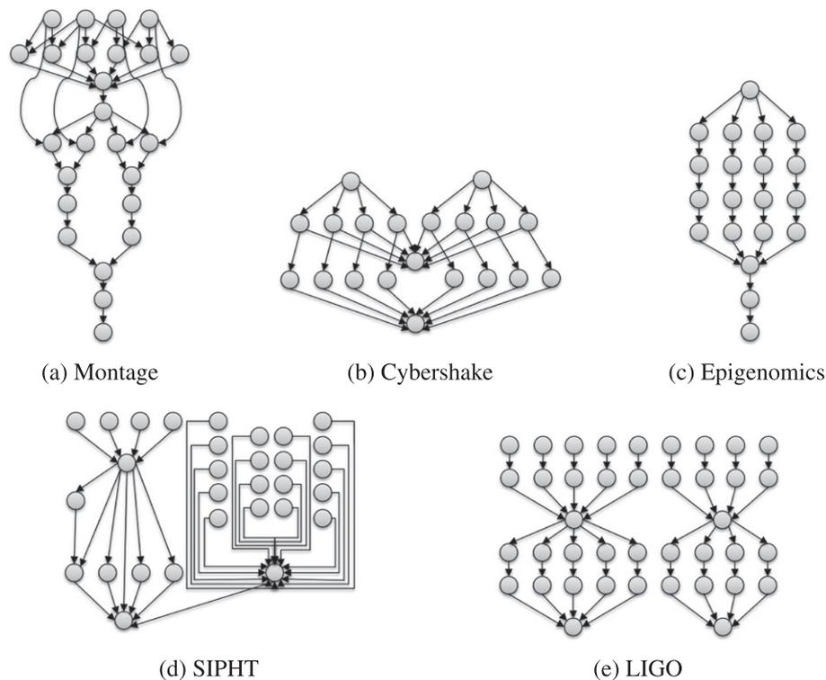
**FIGURE 2** Structure of 5 different scientific workflows: Montage (Astronomy), Cybershake (Earthquake science), Epigenomics (Bioinformatics), SIPHT (Bioinformatics), and LIGO (astrophysics)
