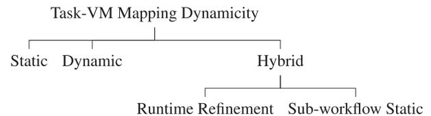
**FIGURE 6** Types of task-VM mapping dynamicality
