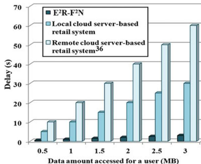
**FIGURE 4** Delay for a user in the proposed energy-efficient retailing using a femtolet-based fog network (E<sup>2</sup>R-F<sup>2</sup>N) and existing cloud server-based retail systems [Colour figure can be viewed at [wileyonlinelibrary.com](http://wileyonlinelibrary.com)]
