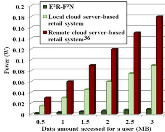
**FIGURE 5** Smart phone's power consumption in the proposed energy-efficient retailing using a femtolet-based fog network (E<sup>2</sup>R-F<sup>2</sup>N) and existing cloud server-based retail systems [Colour figure can be viewed at [wileyonlinelibrary.com](http://wileyonlinelibrary.com)]
