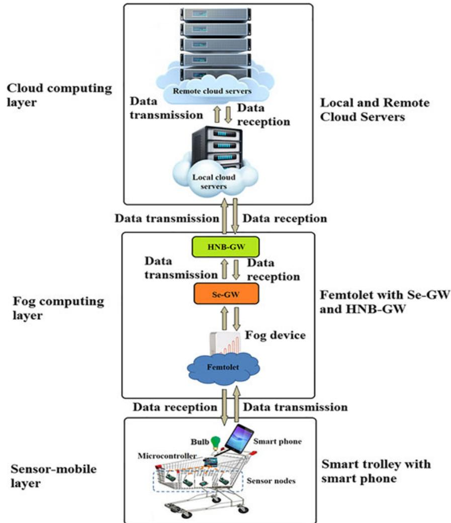
**FIGURE 1** Three-layer architecture of energy-efficient retailing using a femtolet-based fog network. HNB-GW, home node base station-gateway; Se-GW, security-gateway [Colour figure can be viewed at [wileyonlinelibrary.com](http://wileyonlinelibrary.com)]
