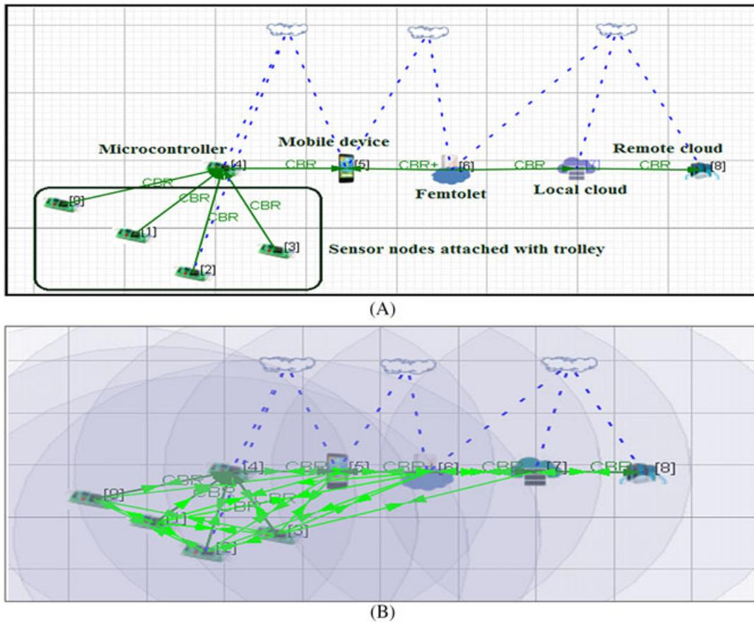
**FIGURE 6** A, Energy-efficient retailing using a femtolet-based fog network scenario created in QualNet 7; B, Simulation scenario during execution [Colour figure can be viewed at [wileyonlinelibrary.com](http://wileyonlinelibrary.com)]
