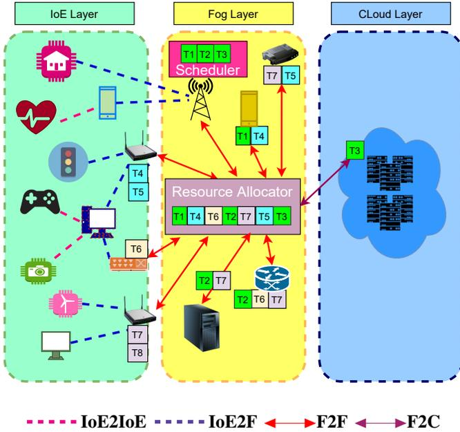
Fig. 1. Fog Computing Architecture. F = Fog Node; C = Cloud; IoE2F = IoE-to-Fog; IoE2IoE = IoE-to-IoE; F2F = Fog-to-Fog; F2C = Fog to Cloud
