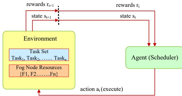
Fig. 6. Reinforcement Learning Architecture.
