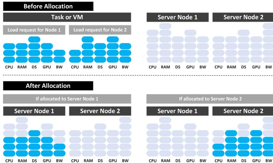
Fig. 2. Allocation of a task or VM to heterogeneous nodes with multi-dimensional resources.
