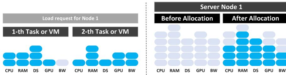
Fig. 3. Relationship of linearly superposition for multi-dimensional resources allocating two tasks or VMs to one server node.
