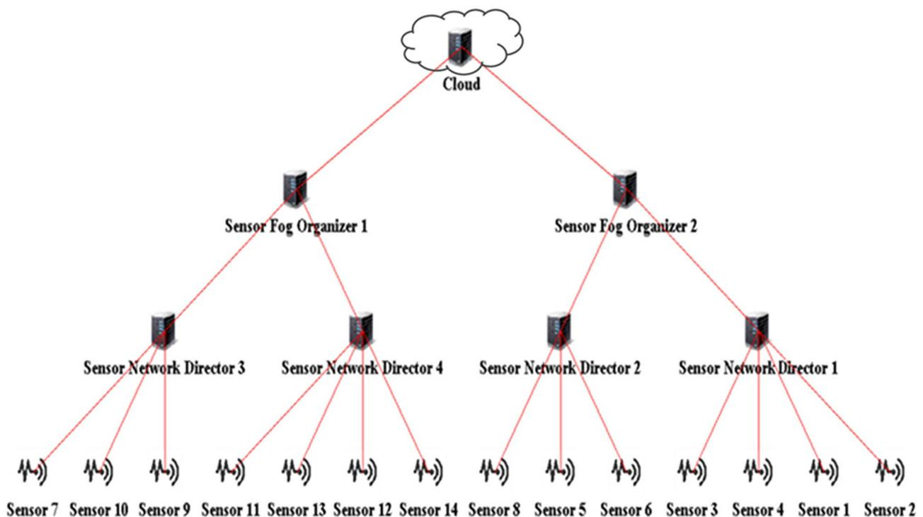
Fig. 2 Created topology of the proposed multi-sensor geo-fog paradigm in iFogSim
