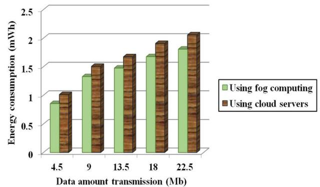
**Fig. 11** Energy consumption of proposed multi-sensor geo-fog network and sensor cloud network
