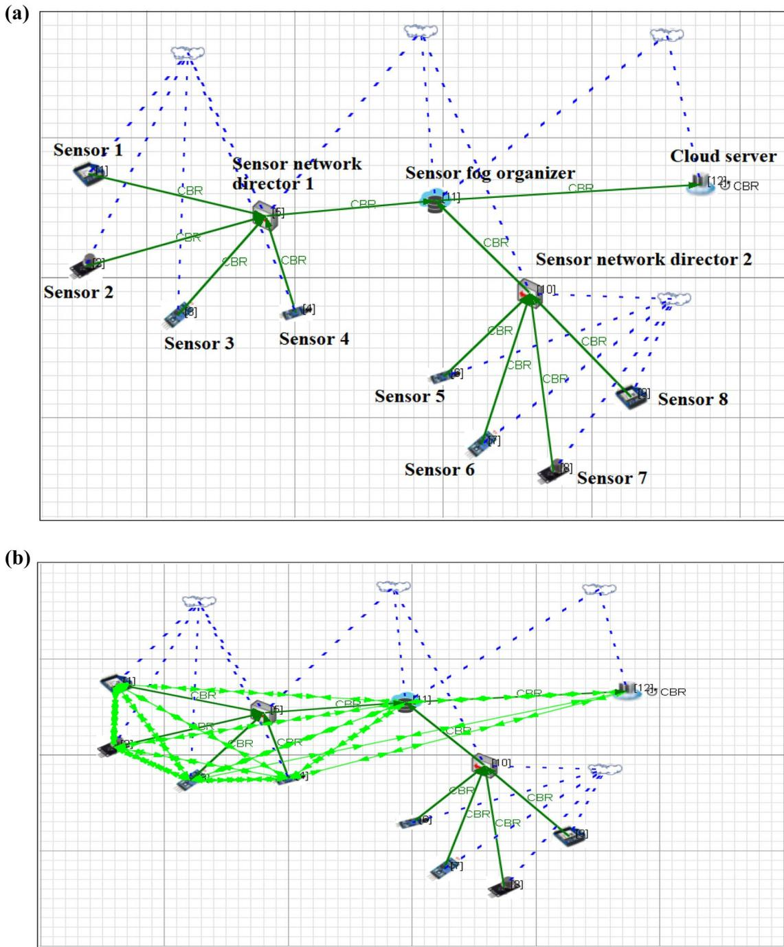
**Fig. 7** a Simulation scenario of proposed multi-sensor geo-fog network for defense sector. b Simulated multi-sensor geo-fog network for defense sector during execution
