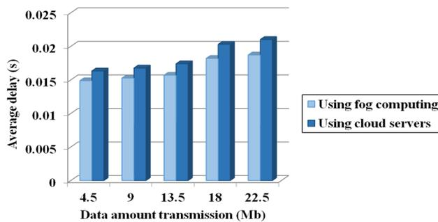
**Fig. 9** Average delay of proposed multi-sensor geo-fog network and sensor cloud network
