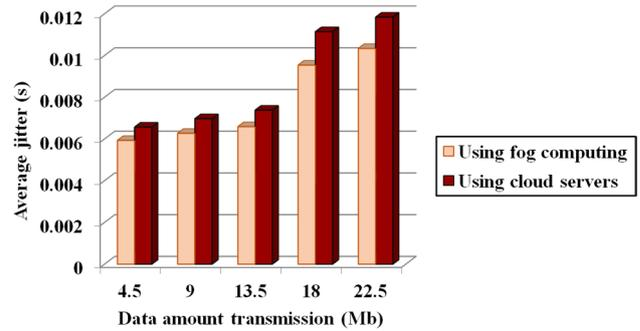
**Fig. 10** Average jitter of proposed multi-sensor geo-fog network and sensor cloud network
