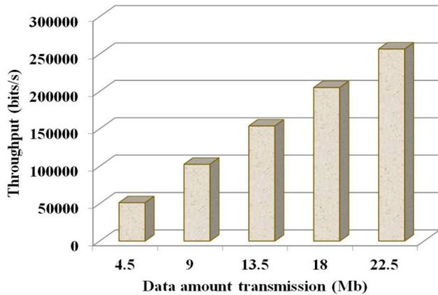
**Fig. 8** Throughput of the proposed multi-sensor geo-fog network
