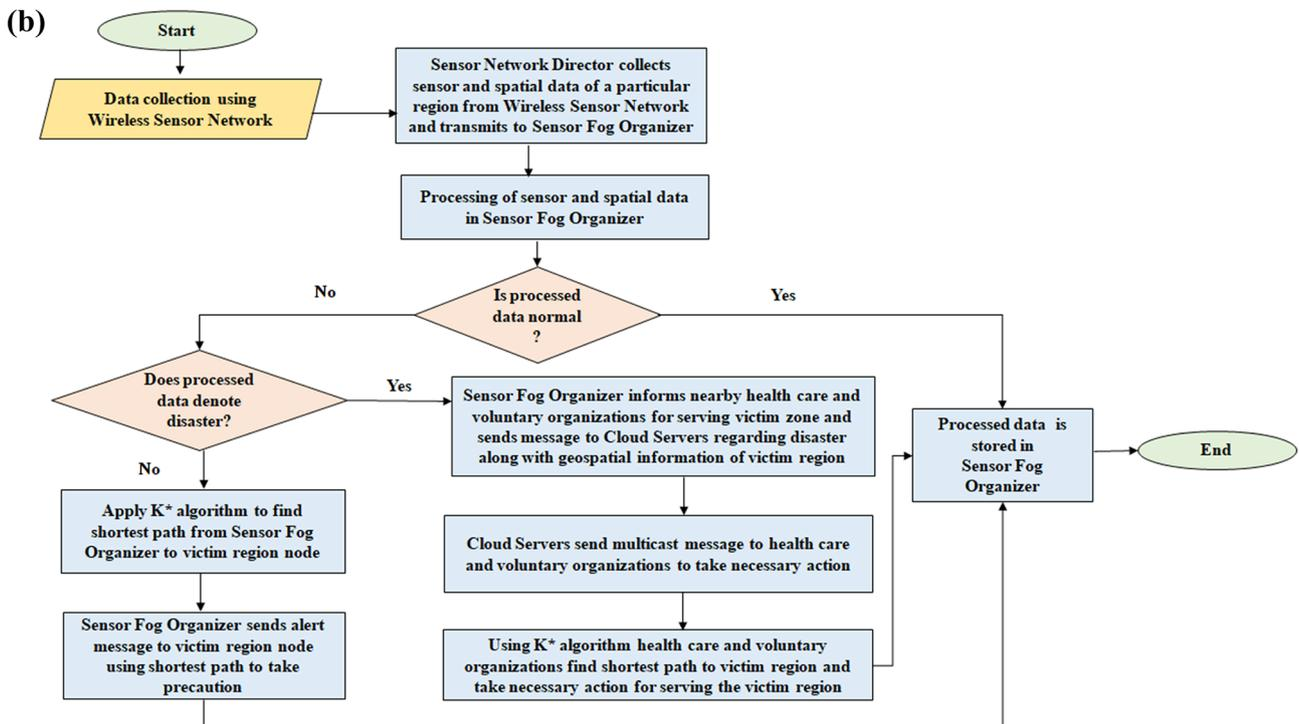
Fig. 1 a Proposed four-layer multi-sensor geo-fog paradigm for defense sector. b A flowchart of the working model of proposed paradigm
