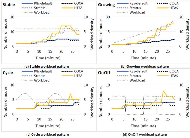
Fig. 5. Number of active worker nodes in response to the workload over time.
