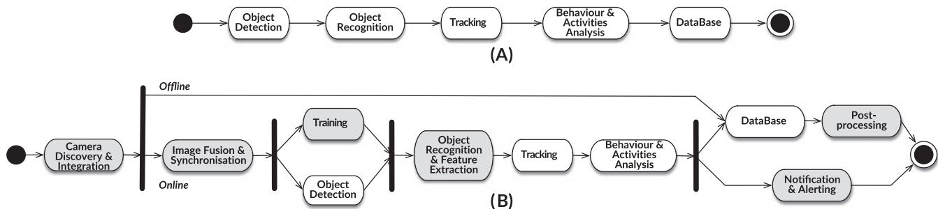
**FIGURE 4** (A) Intelligent surveillance systems and (B) metropolitan intelligent surveillance system reference workflows
