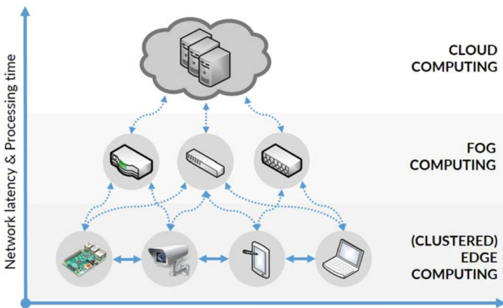
**FIGURE 3** Clustered edge computing and horizontal off-loading [Colour figure can be viewed at [wileyonlinelibrary.com](http://wileyonlinelibrary.com)]
