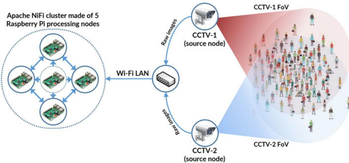
**FIGURE 8** A metropolitan intelligent surveillance system scenario implemented by clustered edge computing. LAN, local area network [Colour figure can be viewed at [wileyonlinelibrary.com](http://wileyonlinelibrary.com)]
