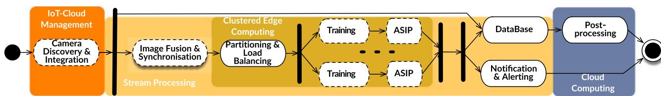
**FIGURE 5** Convergence of IoT-Cloud management, clustered edge computing, stream processing, and cloud computing to enable the MISS reference workflow [Colour figure can be viewed at [wileyonlinelibrary.com](http://wileyonlinelibrary.com)]
