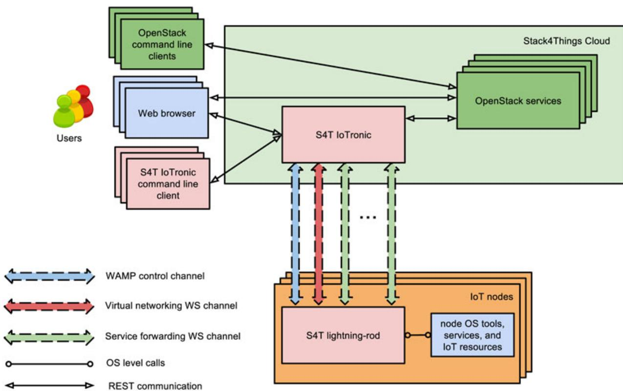
**FIGURE 2** A bird's eye view on the Stack4Things (S4T) architecture. IoT, Internet of Things; REST, Representational State Transfer; WAMP, Web Application Messaging Protocol; WS, WebSocket [Colour figure can be viewed at [wileyonlinelibrary.com](http://wileyonlinelibrary.com)]
