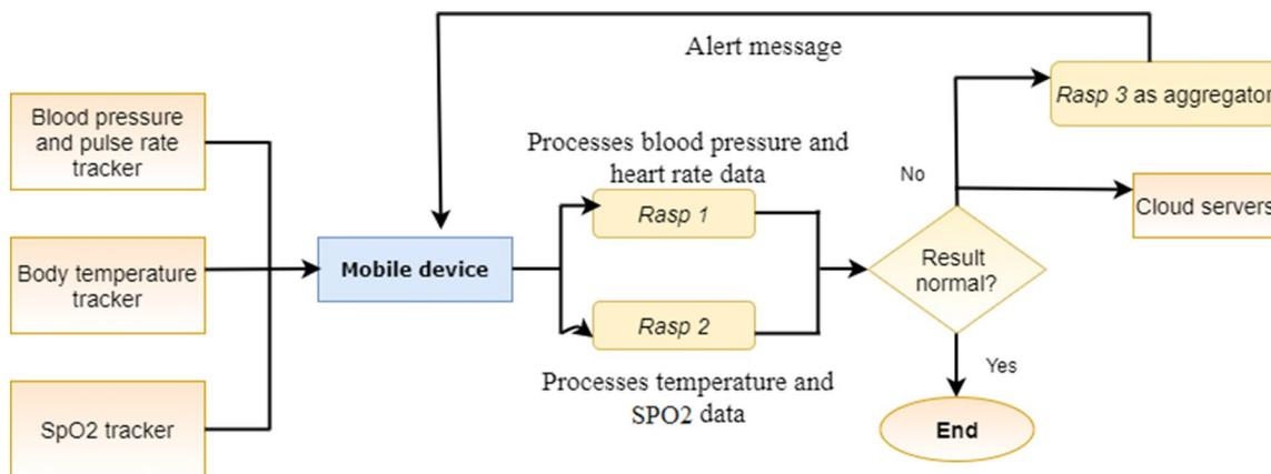
Fig. 9 Data flow diagram of the implemented IoHT framework
