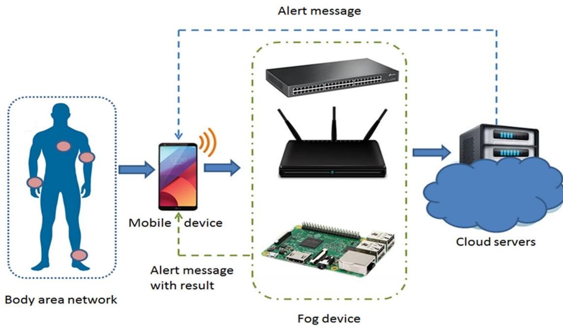
Fig. 1 Edge-fog-cloud based IoHT framework
