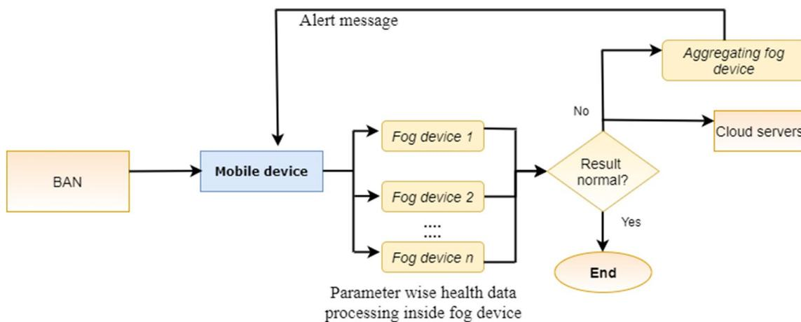
Fig. 2 Data flow diagram of the proposed IoHT framework
