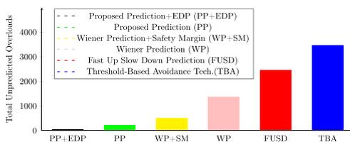
Fig. 9. Comparison of total number of unpredicted overloads during entire testing period.
