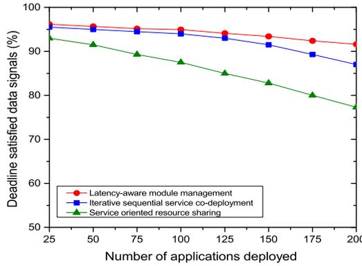
Fig. 5. Percentage of QoS satisfied data signals vs number of applications.
