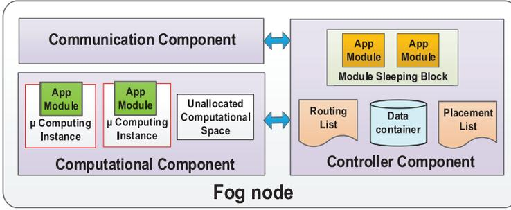
Fig. 3. Fog node components.
