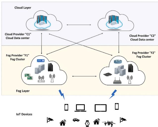
Fig. 1. Federated multi-fog and multi-cloud architecture.
