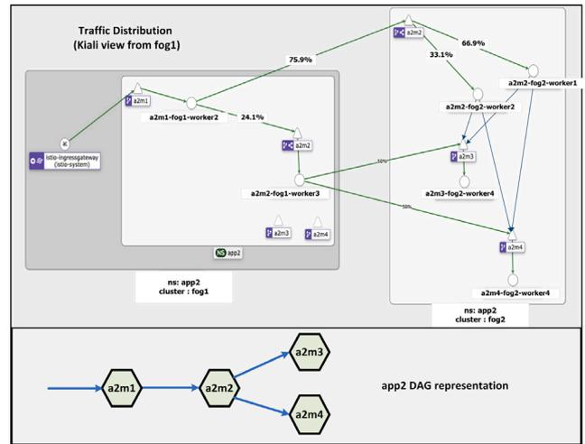
Fig. 15. Multi-cluster service discovery and load balancing scenario - app2.
