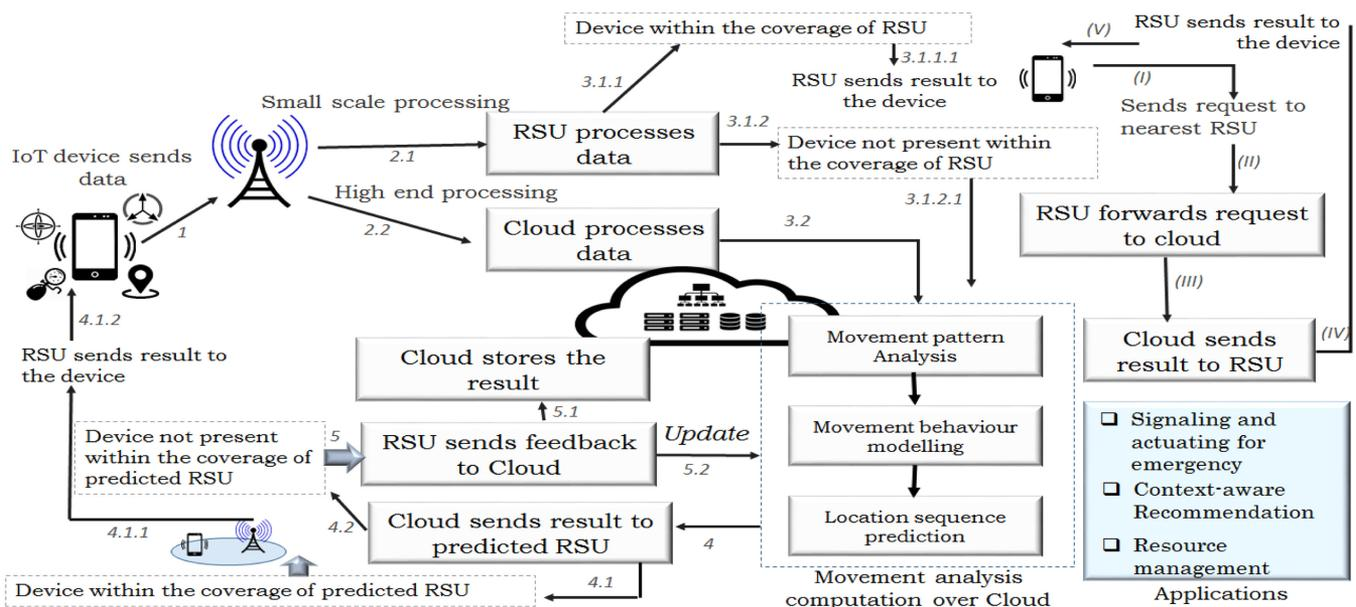
Fig. 3. Working model of the proposed framework, *Mobi-IoST*.
