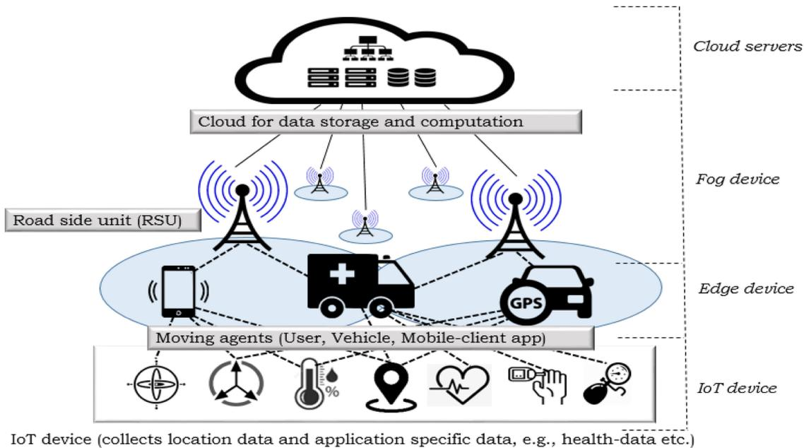
Fig. 2. Hierarchical placement of IoT, Edge, Fog devices and Cloud in *Mobi-IoST* framework.
