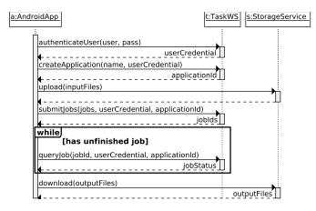
Fig. 4. Basic lifecycle for a mobile application using Aneka.
