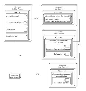
Fig. 2. Deployment Diagram showing how the different artifacts can be deployed and how they communicate.
