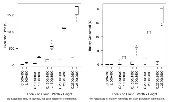
Fig. 9. Boxplot graphs comparing the results for Local and on Cloud execution with different image resolutions: 500x500, 1000x1000, 1500x1500, 2000x2000 and 2500x2500. Each combination of parameters was executed 5 times.
