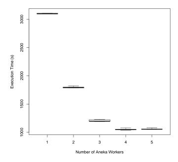
Fig. 10. Boxplot graph comparing the impact of the number of Aneka Workers on execution time. The image resolution is fixed to 12500x12500 and the image generation was split in 25 jobs.
