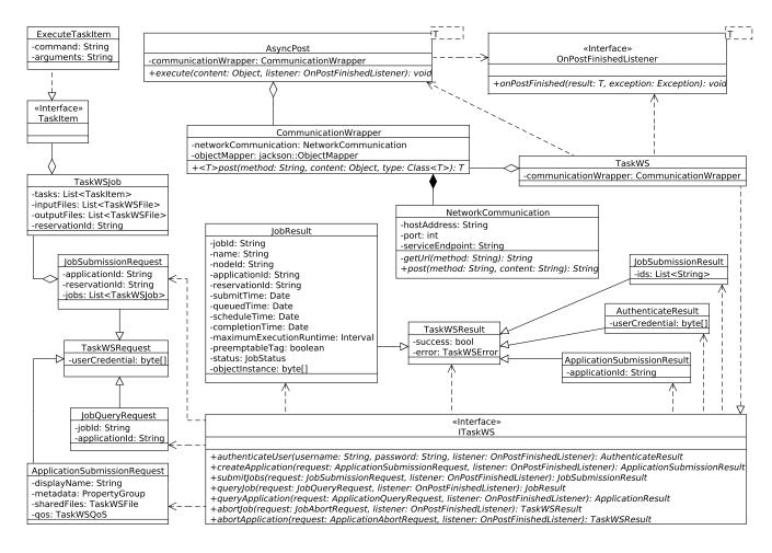
Fig. 3. Class Diagram showing the main classes and interfaces, such as TaskWS and ITaskWS, and how they interact.
