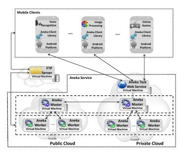
Fig. 1. Architecture showing how mobile devices interact with an Aneka cloud through the *Aneka Task Web Service* in order to outsource resource-intensive tasks.
