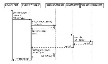
Fig. 6. Sequence diagram for CommunicationWrapper class post method.
