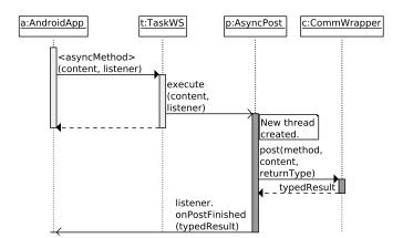
Fig. 5. Sequence diagram for asynchronous methods.
