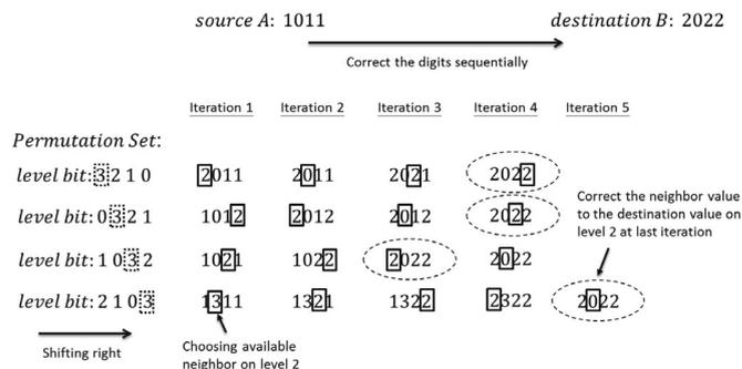
Fig. 2. BSR generates a parallel path set with  $A$  and  $B$ .
