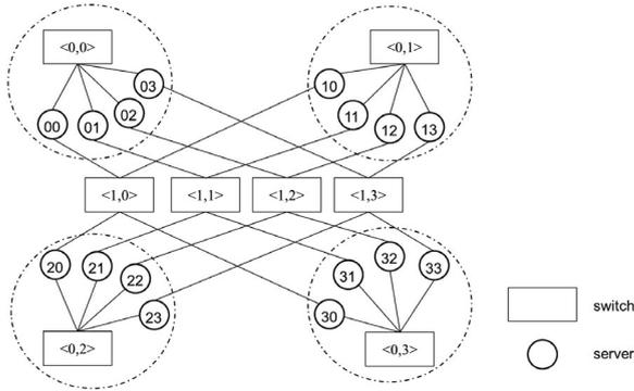
Fig. 1.  $BCube(n, k)$  where  $k = 1$  and switch port  $n = 4$ , each server has  $k + 1 = 2$  ports.
