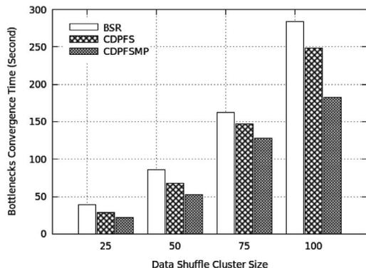
(b) Bottleneck convergence time with different cluster size in data shuffle
