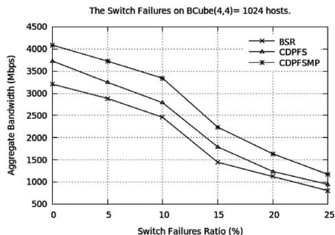
(a) Failure of switches
