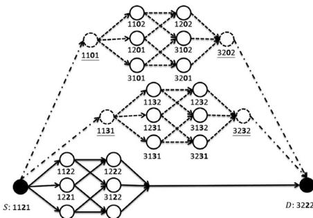
Fig. 5. NSP graph of  $BCube(n, k)$  where  $k = 3$ ,  $n = 4$ ,  $sp_{count} = 3$  and NSP level bit  $j = 1$ . Bit value 1 is not available, and bit value 0 and 3 are chose.
