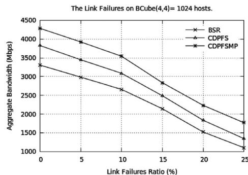
(b) Failure of links
