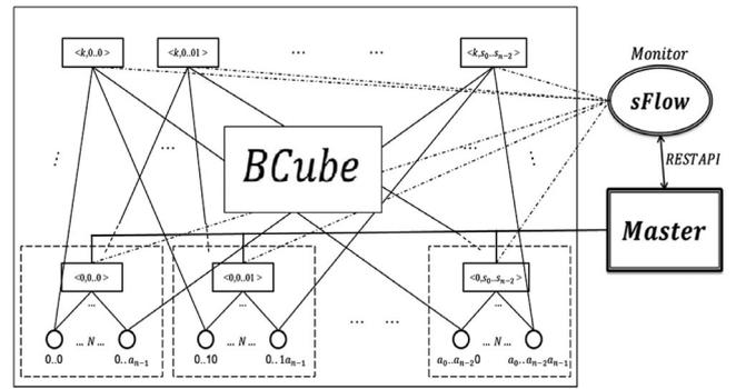
Fig. 10. The Architecture of  $BCube(n, k)$  with Master (Large Parallel Computing Computer) and Monitor (sFlow).
