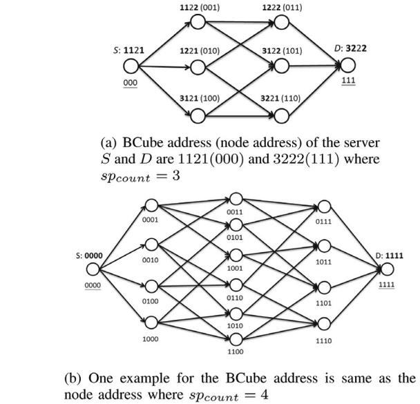
Fig. 3. SP Graph with BCube Address and node address between the server  $S$  and  $D$  in  $BCube(n, k)$  where  $k = 3$  and  $n = 4$ .
