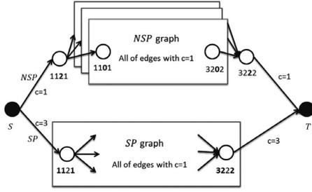
Fig. 8. Flow network with all vertices in SP and NSP graph with  $MPathSet_i$  of  $(S_i, D_i) = (1121, 3222)$ .
