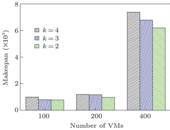
Fig.10. Comparison of time costs for PrepartitionOn1 by varying values of  $k$ .
