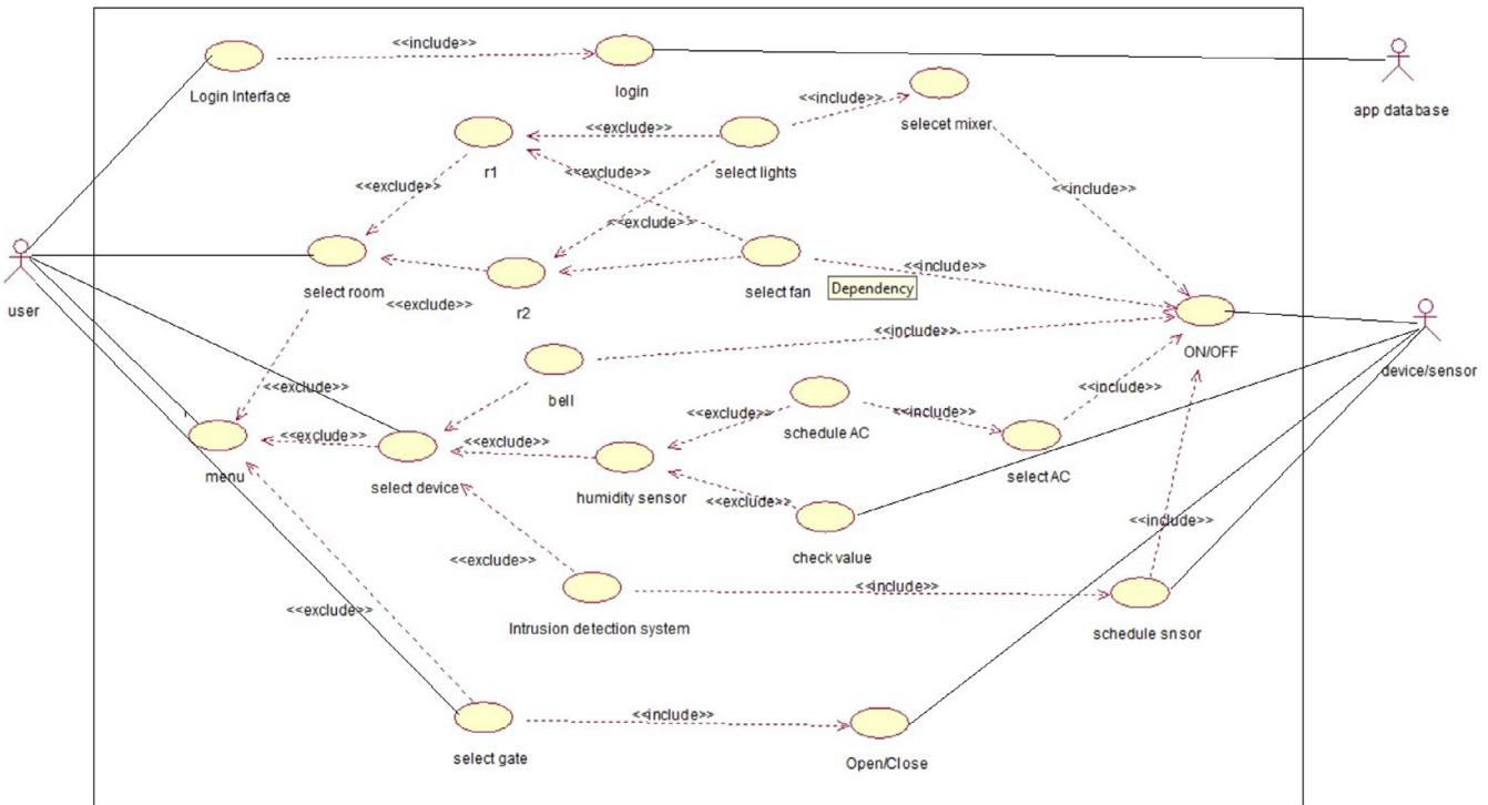
**Fig. 9.** Use Case Diagram of Smart Home Automation.
