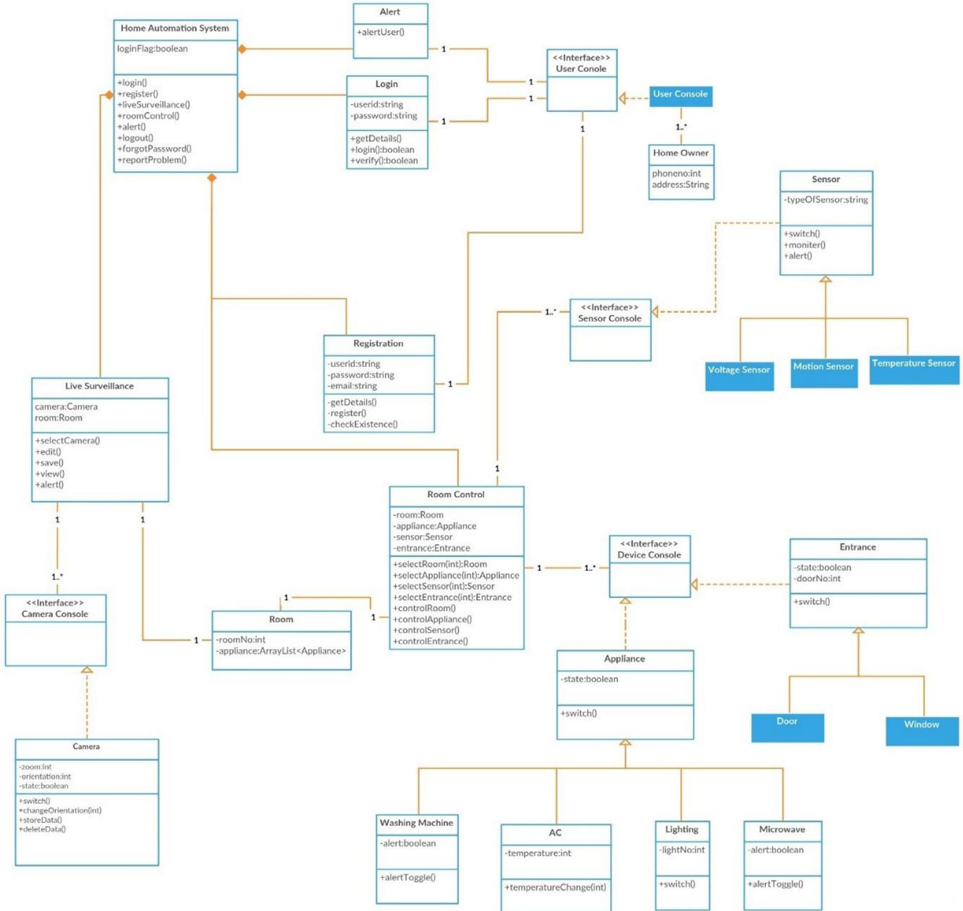
Fig. 10. Class Diagram of Smart Home Automation.
