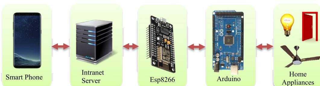
**Fig. 7.** Interaction of Different Components.
