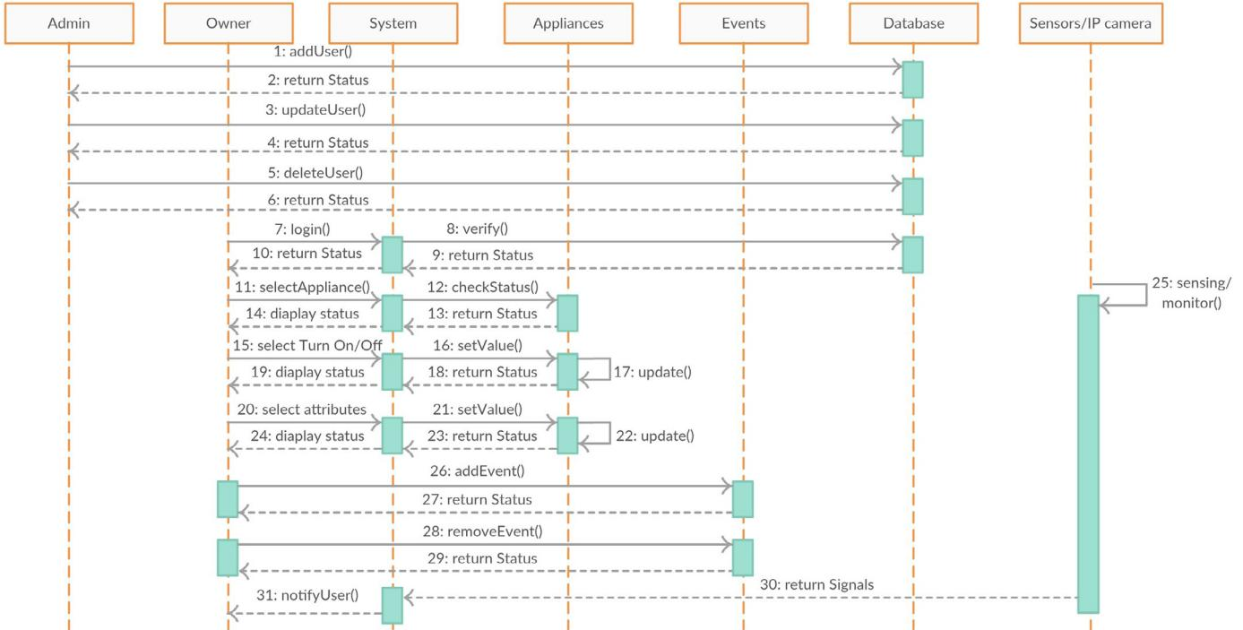
**Fig. 12.** Application Model of the Smart Home Automation.
