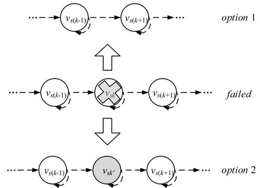
Fig. 16. State recovery for a failed stateful vertex.
