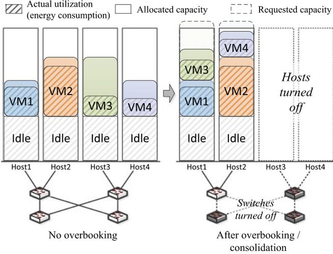
Fig. 2. Example of consolidation with overbooking.
