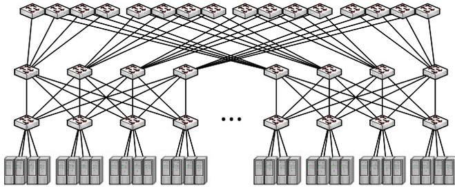
Fig. 3. Network topology used in simulation.
