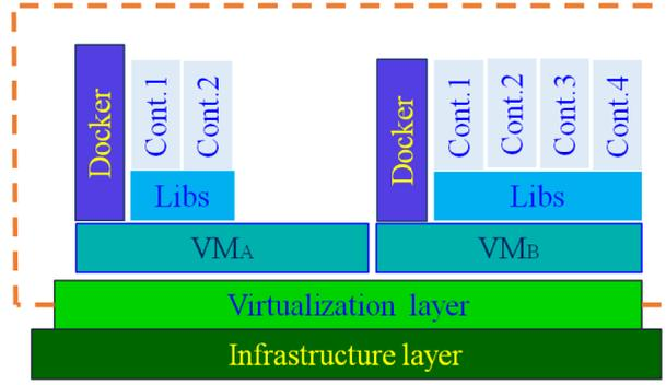
Fig. 3. Virtualized environment in container CloudSim [3]
