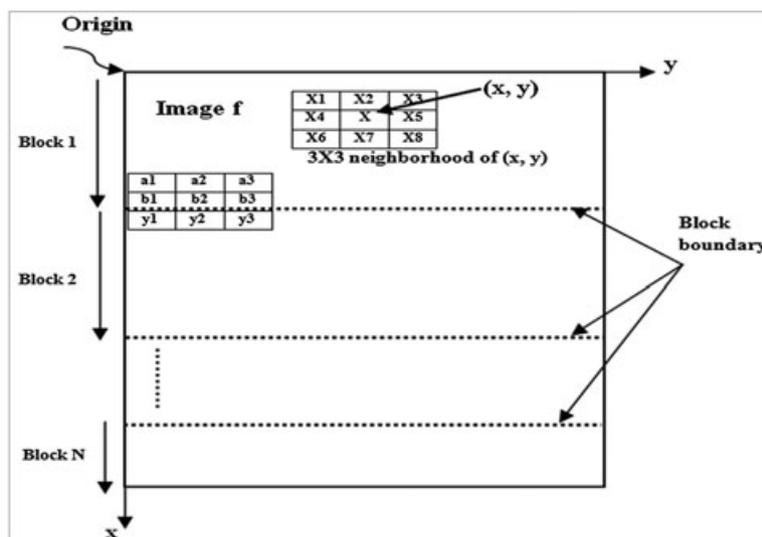
Figure 1. Image representation with segmented blocks.
