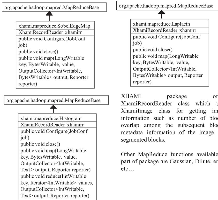
Figure 5. XHAMI MapReduce package for image processing domain.
