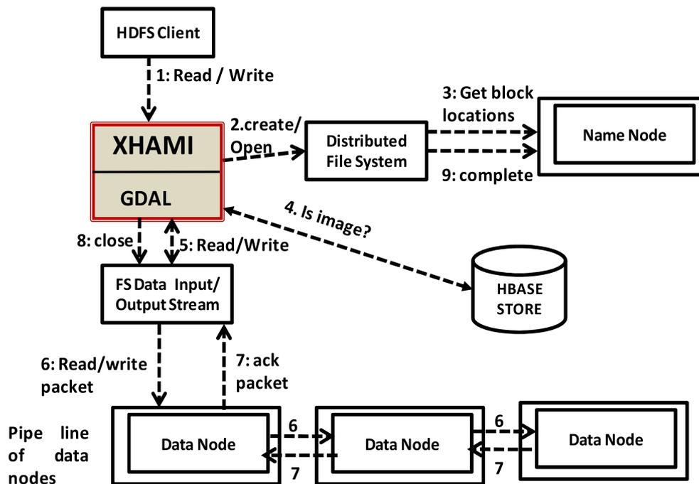
Figure 2. XHAMI for read/write operations.
