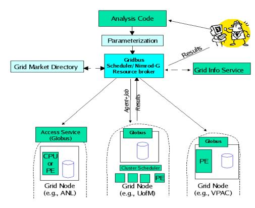
Figure 2. Architecture of brain-activity analysis on the Grid.
