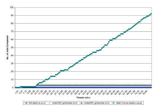
Figure 8. Scheduling with cost optimization: cumulative graph of the number of jobs completed versus time.
